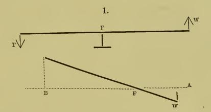
consists of a rigid rod, movable upwards and downwards only, on a given point, which is called a *fulcrum*. At the one extremity of the rod a certain power is exerted, at the other is the weight to be raised, or the body to be influenced.
